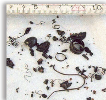
DEBRIS COLLECTED AND REMOVED FROM AN OPERATING BWR
